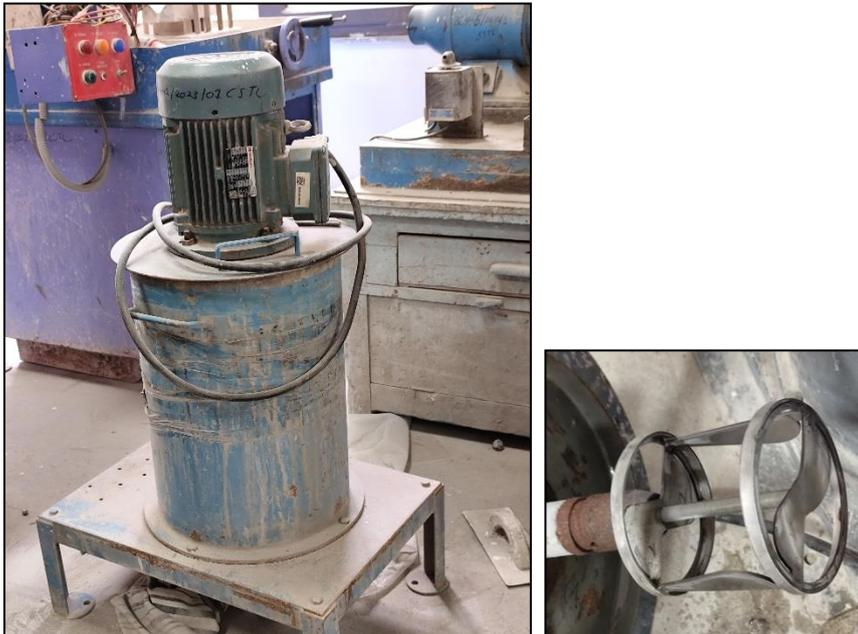
**Figure 2.** Test Setup according to ASTM C1138 [4]
