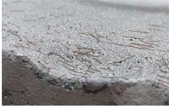
**Figure 3.** Indentations caused by high speed steel balls
