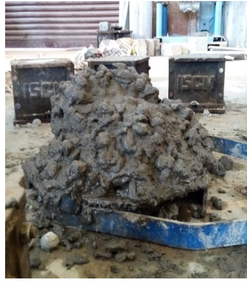
Fig.14 Shear collapse for 25% slag + 25% fly ash
