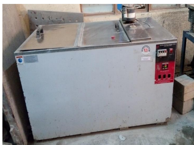
Fig.18 Accelerated curing tank
