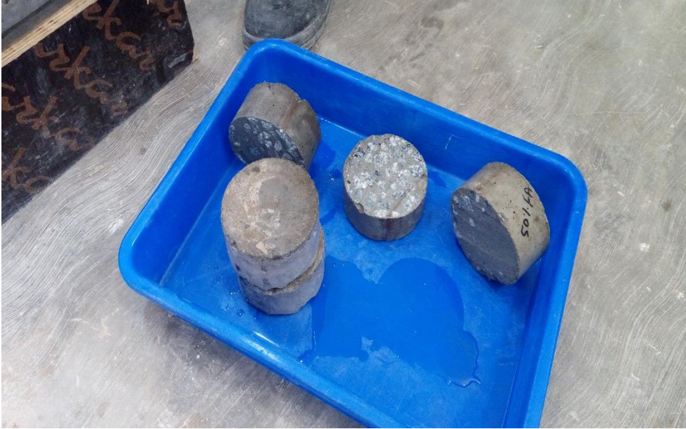
Fig.19 Concrete cylinders cast for Rapid Chloride Penetration Test
