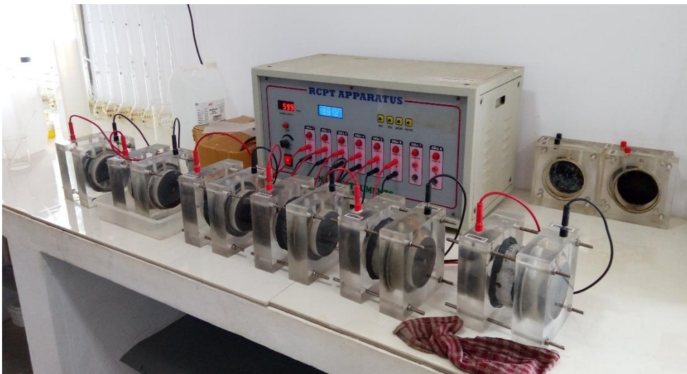
Fig.20 Rapid Chloride Penetration Test Apparatus
