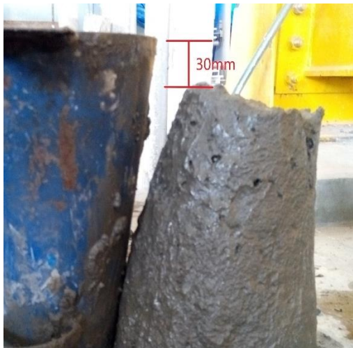
Fig.15 30mm slump for 25% slag + 10% Silica fume
