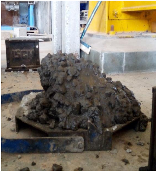
Fig.13 Shear collapse for 50% Slag
