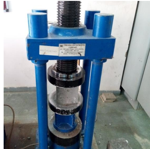
Fig.16 Compressive strength test on cubes
